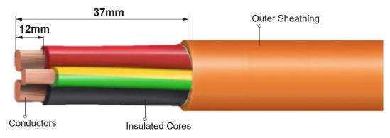
Figure 3: Cable Stripping Lengths
